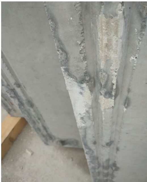
防滑条脱模时破损
